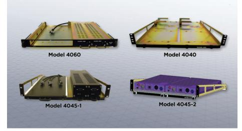
Model 4060 provides power and effortless slide rail access for installation and removal of one KG-350 encryption device. Model 4045 also provides power and mounting for up to three KG-350s (with optional 4045-2 daughter rack) and is designed to operate in severe environmental conditions. Model 4040 is designed to securely mount up to two KG-350s and power bricks.
